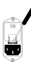
1: Insert a small screwdriver into the hook beneath the fuse sled and pull it out from its retaining clip. Hold the hook with your fingers and gently pull the sled out.
